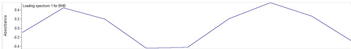
Figure 13 Loading spectrum 1 of the PLS model for BHB developed using spectra collected on prototype 3. Two peaks are
