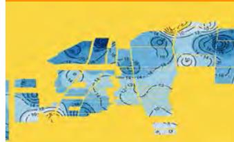
Maps of soil water availability for plants are a tool for precision irrigation management, allowing the growers to save water and apply an accurate amount of water in appropriate areas.
