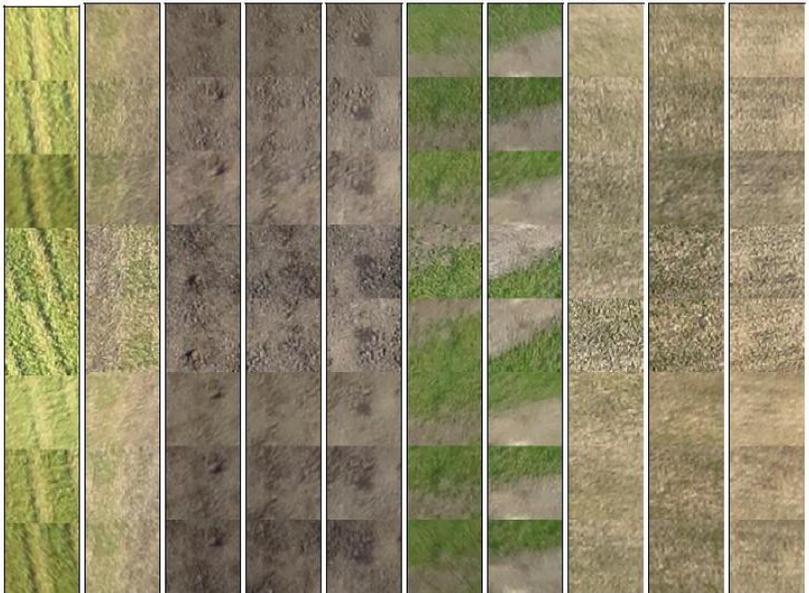
Figure 6: Cropped area of 10 3D points arising from 8 2D keypoints. Each cropped area should represent the same object on the ground.
